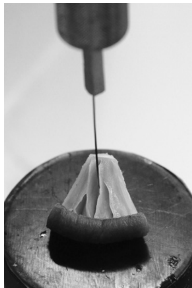
Fig. 2. Needle insertion test with EZ-Test. The energy necessary to penetrate a remoistened shiitake cap with a needle (0.2mm in diameter) was determined.
